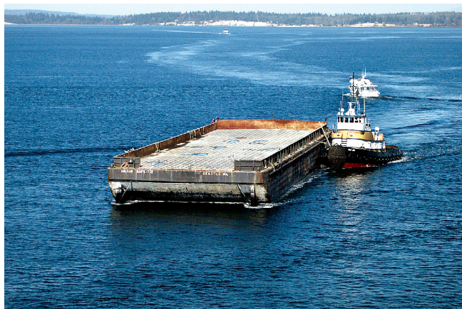
All barges would go under the eastern span (Kitsap end) of the Hood Canal Bridge. A tug and typical-sized, 60-foot-wide barge (left and above) navigate the 230-foot opening.
