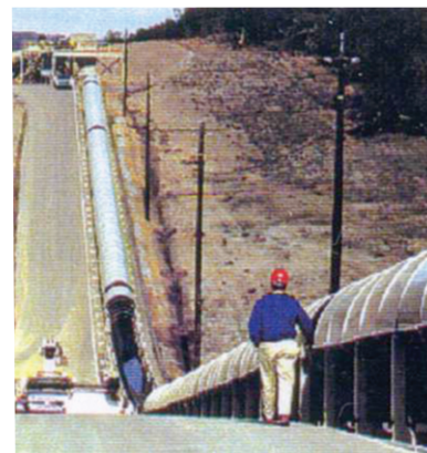
A covered conveyor similar in design to the Central Conveyor half-moon cover.
